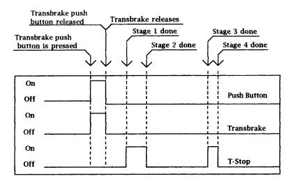
NOTE: The 4-Stage Timer can also be used to control other timed devices, nitrous, or timing retards.
