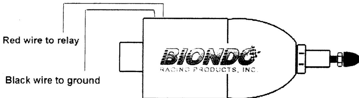
When hooking up this solenoid to our Mega Series delay box or one of Biondo's shift boxes, follow this diagram.
