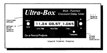
Liquid Crystal Display: This is a 16 character by 1 line display which is has a soft green back light for easy night time viewing. All information about Delay, Dialins, and features is displayed here.
