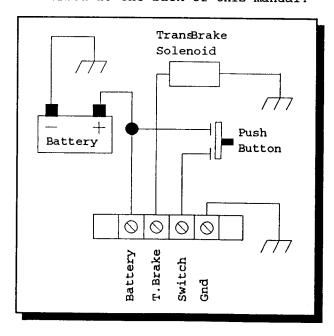
Output Short Circuit Protection: The box has a built in short circuit protection feature. If an electrical short develops in the transbrake solenoid, or in the wiring from the box to the solenoid, the message
