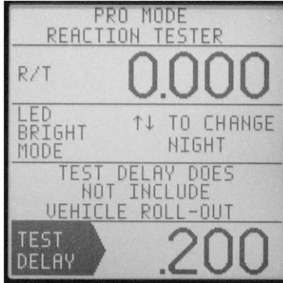
The Driver's Reaction Tester has been improved in the Elite 700 to allow the driver to practice using a pro tree. This allows the driver to practice releasing the button off a pro tree. To do this required an addition of a practice delay time called Test Delay. The Test Delay only affects this screen.
