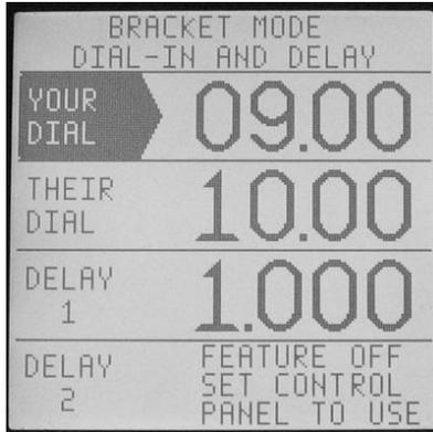
To use the features of the Elite 700, information needs to be entered. Information is entered using the keypad and is shown on the screen. There are three groups of screens; the Control Panel screens (set up first), Bracket Mode screens, and Pro Mode screens.
