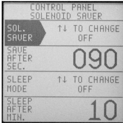
The Solenoid Saver feature keeps the Transbrake solenoid from being destroyed when a button is accidentally left locked on. Using times of 60 seconds or more is recommended.
