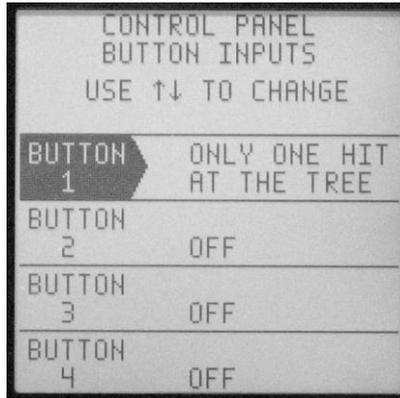
Enter your Button selections first here, and then wire the corresponding Push-buttons to the matching P.B. terminals on the Relay Board.
