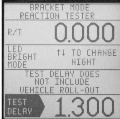
The Driver's Reaction Tester has been improved in the Elite 700 to allow the driver to practice using a full tree. This allows the driver to practice releasing the button off any bulb. To do this required an addition of a practice delay time called Test Delay. The Test Delay only affects this screen.
