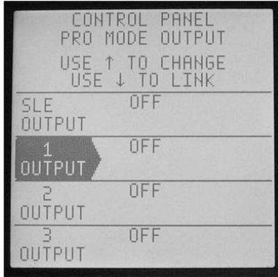
Enter your Pro Output selections first here, and then wire the corresponding devices to the matching Pro Output terminals on the Relay Board.
