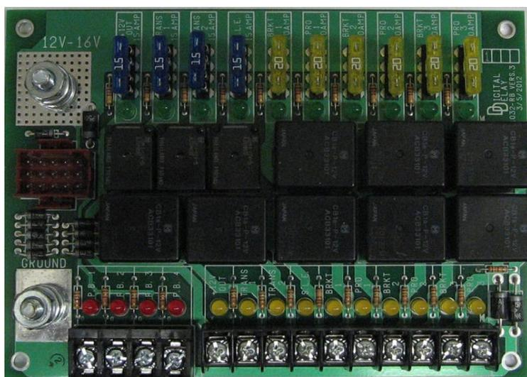
**The Relay Board is where all the electrical connections are made.** The plug from Elite 700 plugs into the same-colored socket on the Relay board, it will only fit in one way. This is the only connection that is necessary between the two. The Relay Board has two power studs, one for ground and one for power. It also has four push-button inputs and 10 fused outputs.
