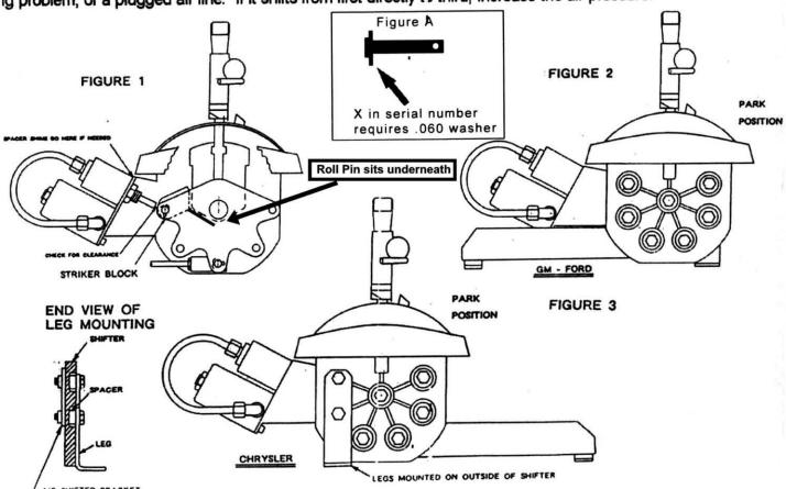
NOTE: THE ROLL PIN STICKING OUT OF THE STRIKER BLOCK DOES "NOT" GO IN THE HOLE ON THE BACK OF SHIFTER HANDLE. BLOCK IS MADE TO BE FLUSH ON THE RAIL.
