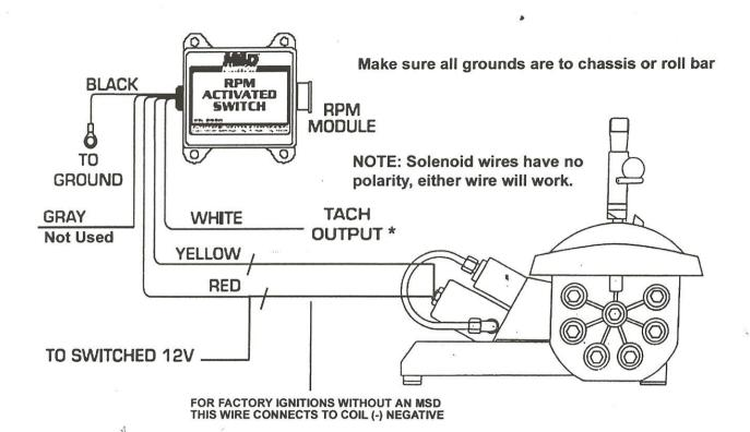
Switch must be turned on prior to staging and must be turn off after run. This serves 2 purposes. One, it saves CO2 by not engaging during warm-ups or burnout. Second, and more important it prevents any chance of the car shifting out of neutral during warm-ups which can create a hazardous situation.
